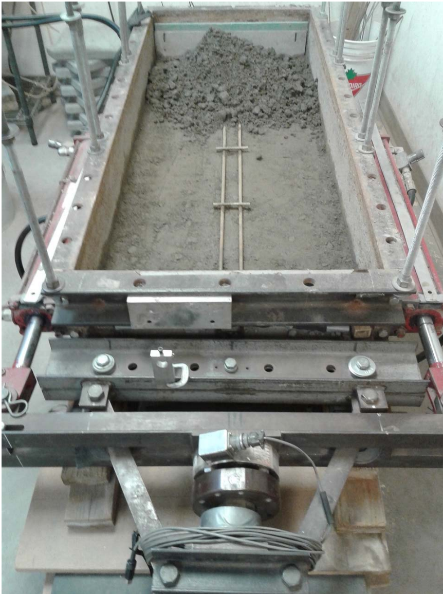
Figure 4. Elevate Ladder Strip placed on compacted GAB material.
