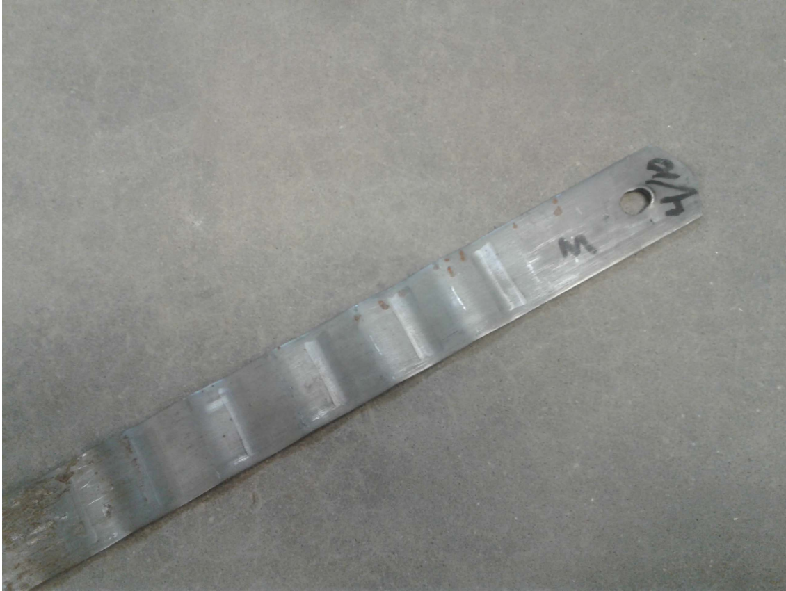
Figure 10. Failure mode: stretching of the Wave Strip connection hole observed at the completion of high pressure (4800 psf) test #3G in AASHTO #57 stone.
