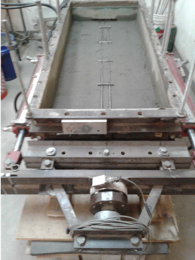
Figure 3. Elevate Ladder Strip placed on compacted sand.
