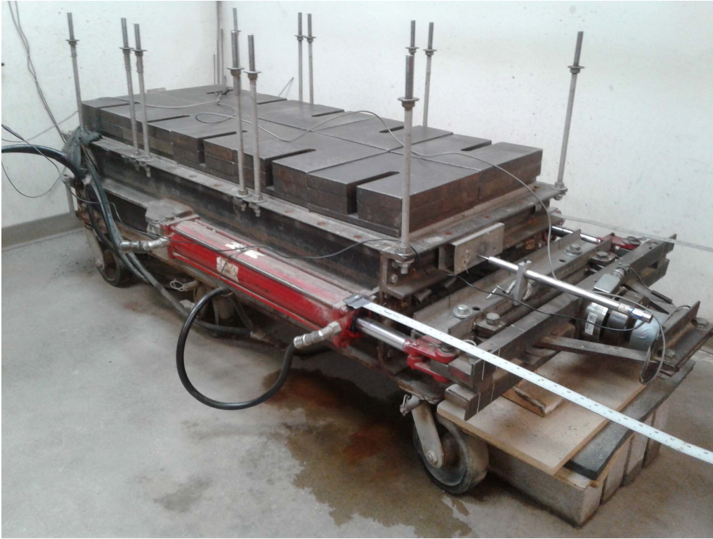
Figure 6. A complete pullout test setup (200 psf normal stress by dead weight).
