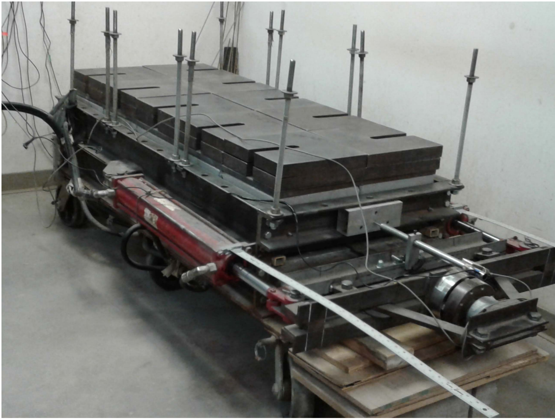
Figure 8. A complete pullout test setup (200 psf normal stress by dead weight).
