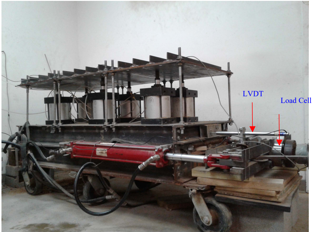
Figure 7. A complete pullout test setup (normal stress by using air cylinders).
