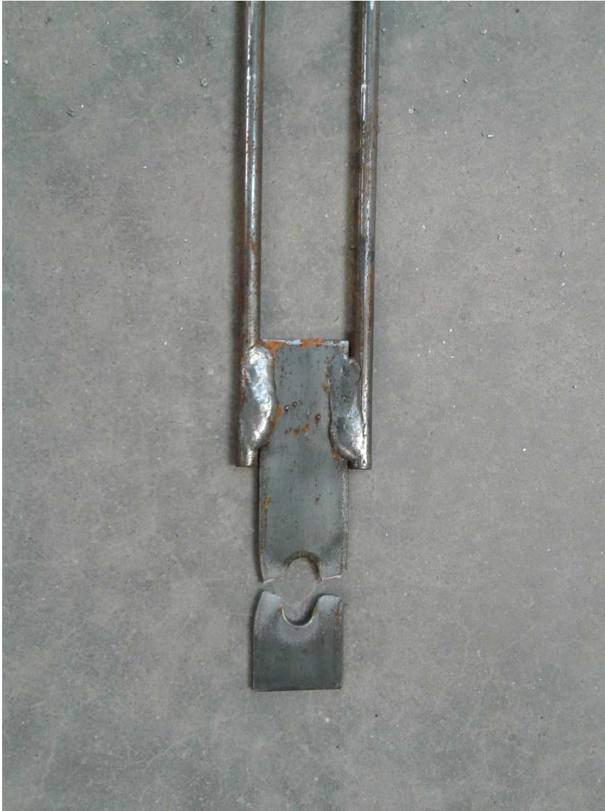
Figure 8. Failure mode: rupture (i.e., tensile failure) of the 1.5 inch wide x 0.18 inch thick connection plate at the connection hole occurred in Tests #2F, 2G, and 3E, 3F, and 3G.
