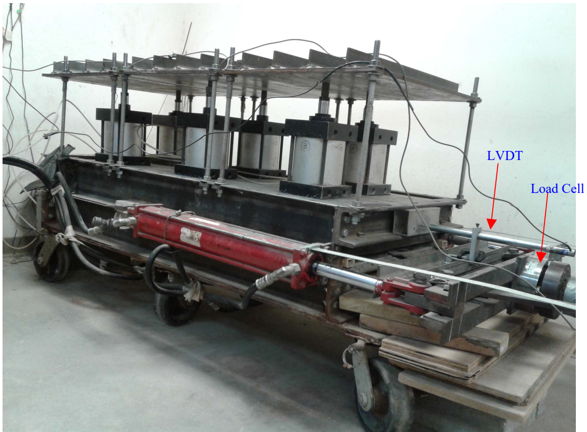
Figure 9. A complete pullout test setup (normal stress by using air cylinders).
