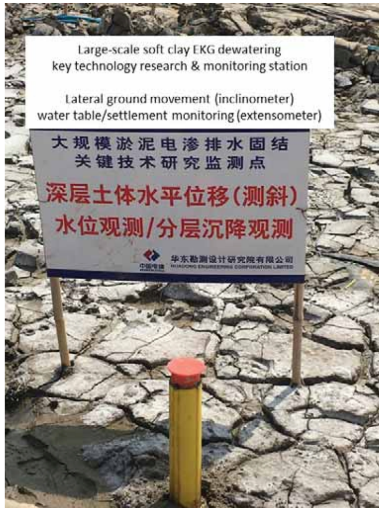
Fig. 9.10. Site instrumentation monitoring lateral and vertical movements, and water table depth.
