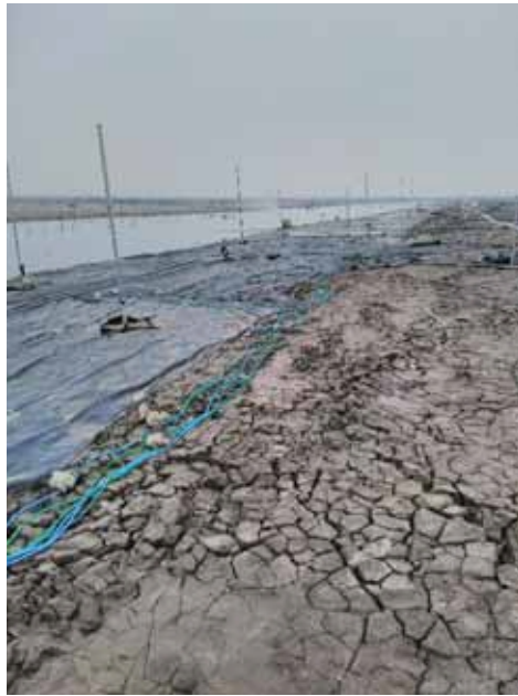
Figure 3 Field trial of soft ground improvement by electro-osmotic consolidation
