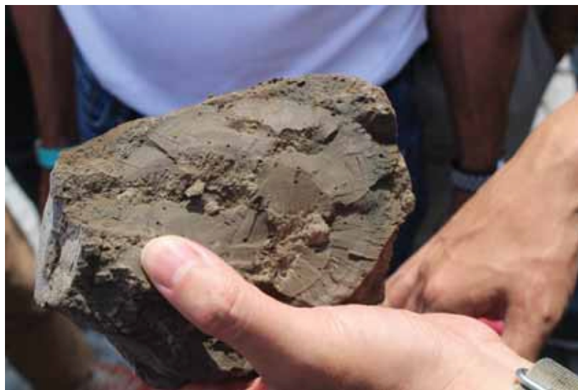
Fig. 10.1 Discoloration through oxidation and tiny wormholes in the silty soils used for the land reclamation in Taizhou affecting the soil behavior
