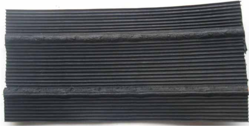
Fig. 9.2. EKG made from conductive polymer (patented in China in 2012).
