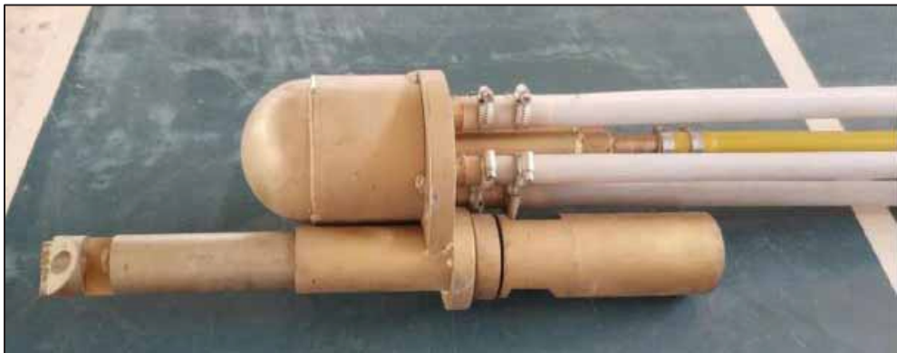
Fig. 4.2. Detachable anchor head (the lower portion is a retractable pushing rod with grout injection port) (source: Zhejiang Zhongqiao Prestress Equipment Co., Ltd. and the Architectural Design and Research Institute of Zhejiang University Co., Ltd.).
