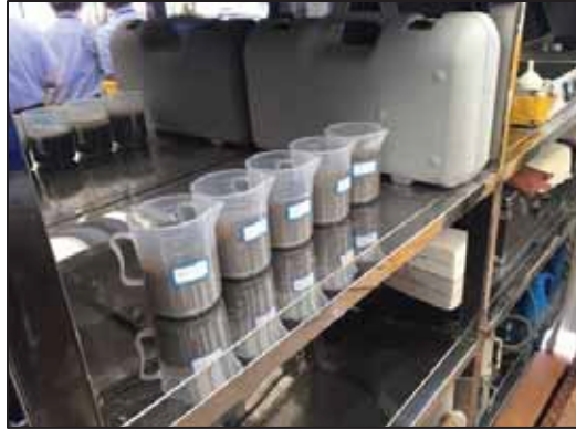
Fig. 2.12. Quality assurance / quality control performed on the bentonite slurry
