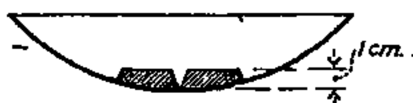
FIG. 3—DETERMINING LIMIT OF LIQUID STATE (ATTERBERG)
